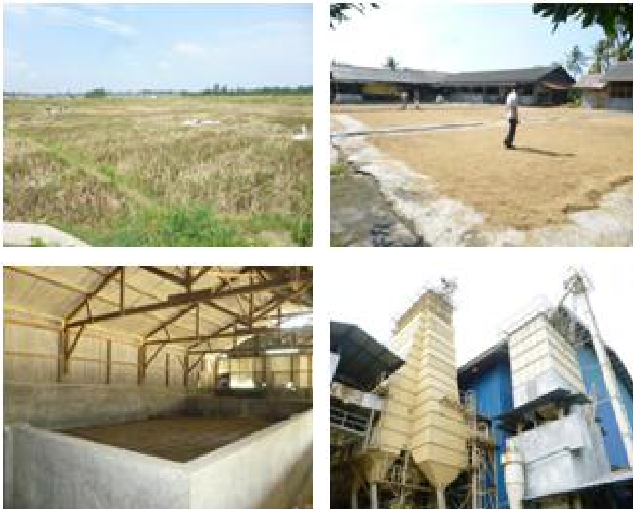
Picture 3-1. Manual harvesting, sun drying, flat bed drying and continuous column drying of paddy in Karawang
