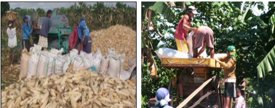
Picture 5-11. Corn shelling with 2 kinds of shellers: hopper at the side and on top
