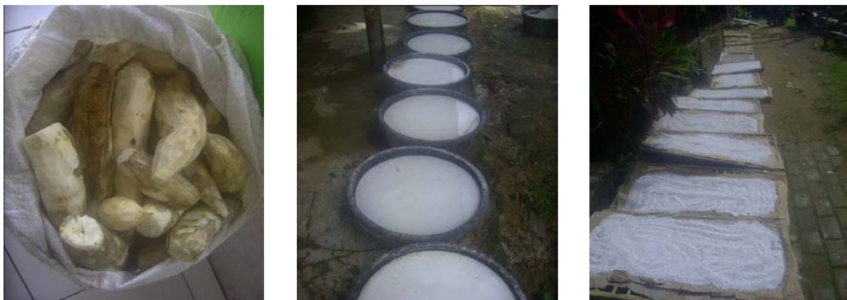
Picture 3-7. Tapioca processing in the home industry: Peeled cassava, settling and sun drying the starch
