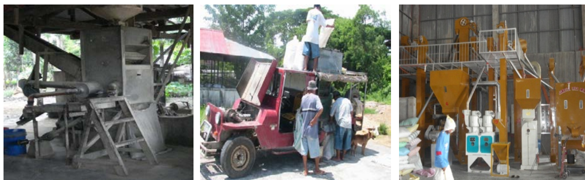
Picture 5-8. Different types of rice mill: stationary single pass, mobile single pass and multi-pass rice mill
