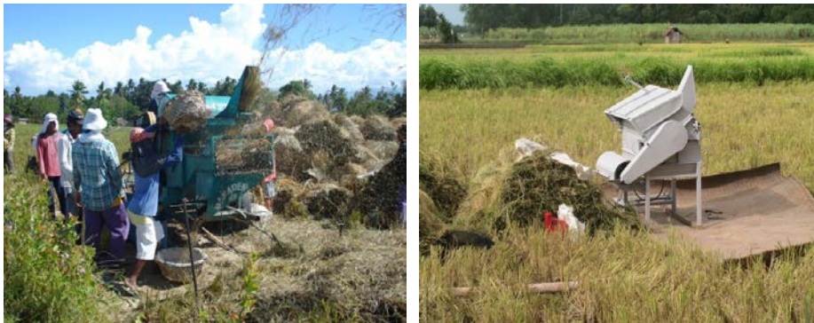
Picture 5-4. Threshing of palay and underlay used to collect scattered and spilled grains
