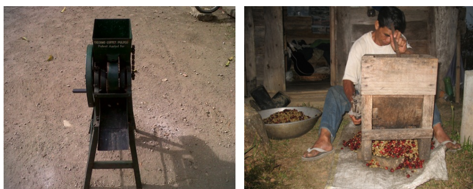
Picture 5-26. Mechanical and wooden depulpers used in wet processing of coffee
